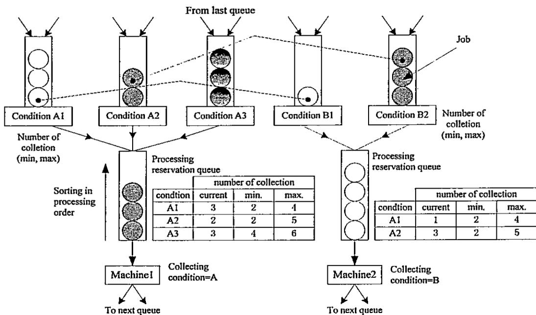
Fig. 1 Hierarchical queue model for lot formation processing
