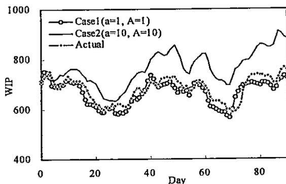
Fig. 3 Total WIP in Cold-Rolling Process
